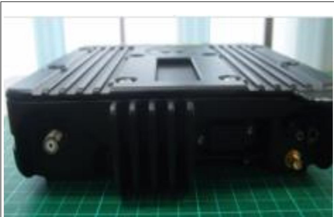
Foto - RF Port/RF Test Point/Interface
